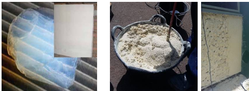
Figure 2. Image of aerogel and aerogel mortar insulation
